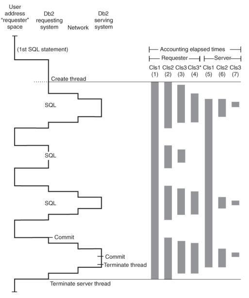
Figure 42. Elapsed times in a DDF environment as reported by Tivoli OMEGAMON XE for Db2 Performance Expert on z/OS
