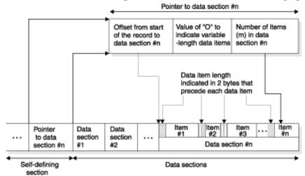
Figure 62. Relationship between self-defining section and data sections for variable-length data items
