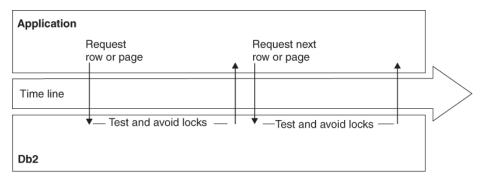
Figure 17. Best case of avoiding locks by using the ISOLATION(CS) and CURRENTDATA(NO) options
