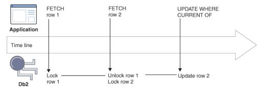
Figure 13. Positioned updates and deletes with a static non-scrollable cursor and without optimistic concurrency control
