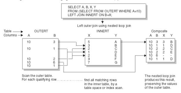
Figure 48. Nested loop join for a left outer join
