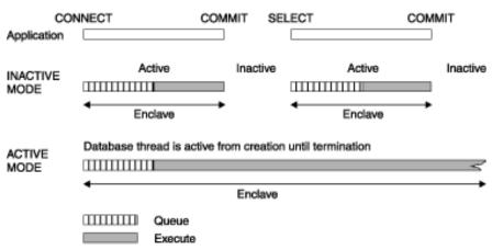
Figure 43. Contrasting ACTIVE MODE threads and POOLED MODE threads
