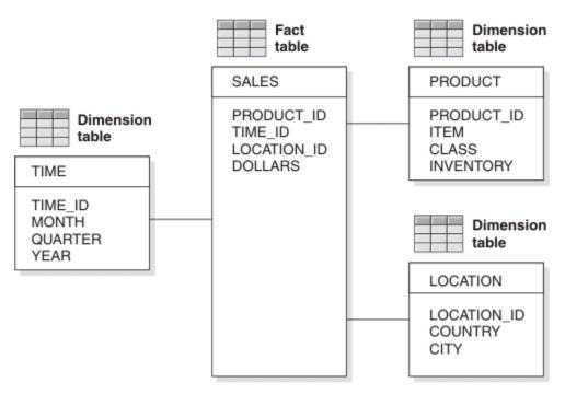
Figure 52. Example star schema with three dimension tables
