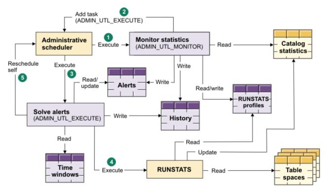
Figure 30. Object interactions for autonomic statistics maintenance in Db2
