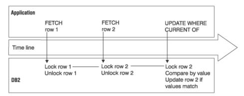
Figure 14. Positioned updates and deletes with a static sensitive scrollable cursor and with optimistic concurrency control
