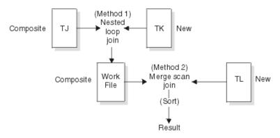
Figure 47. Two-step join operation
