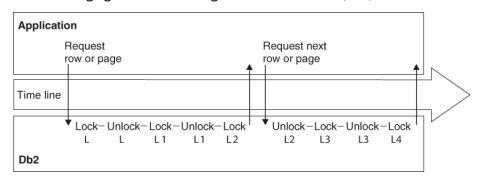
Figure 16. How an application that uses CS isolation with CURRENTDATA (YES) acquires locks
