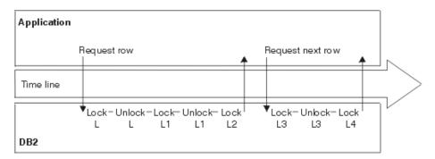
Figure 15. How an application that uses RS isolation acquires locks when no lock avoidance techniques are used
