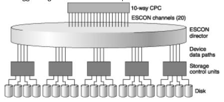
Figure 22. I/O configuration that maximizes performance for an I/O-intensive query
