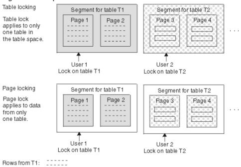
Figure 10. Page locking for simple and segmented table spaces
